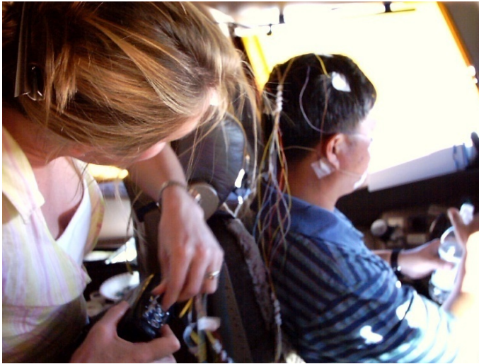
Figure B-10: Polysomnographic recording in flight
